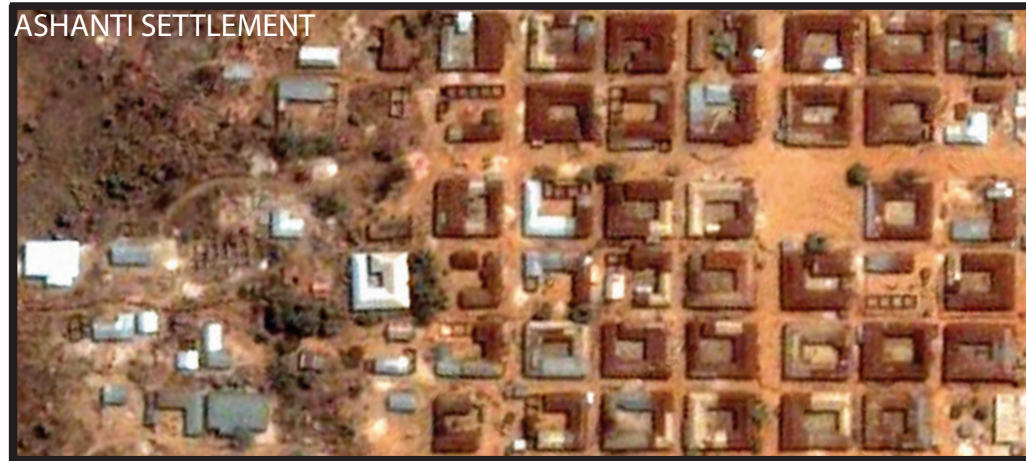
Ashanti Settlement Ghanian settlements emerge little by little in a common urban raster in Ghana - 25m x 30m road axis - 20m x 25m house outlines
